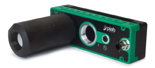
It is available with a three-stage COAX\* cartridge MIDI. Choose an Si cartridge for extra vacuum flow, a Pi cartridge for high performance at low feed pressure or an Xi cartridge when high flow and deep vacuum is needed. This pump has a substantially lower air consumption compare to competition, it is compact with no moving parts. It can be configured with 1–6 cartridges. This pump can easily be upgraded with more capacity if needed. And it is also easy to disassemble for maintenance.
