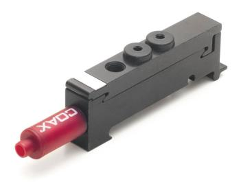
Compact/stackable vacuum pumps are air-driven multistage ejector families, based on COAX® technology, they are equipped with integrated controls and special functions, such as on/off valve, blow-off valve, vacuum switch, energy saving function etc. They are configurable platforms, making it easy to specify the exact control functions needed for the system.
