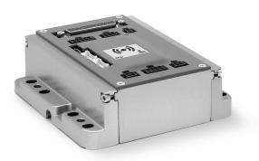
Series DRCS drives, compact and optimised in one size, are capable of controlling all Camozzi Stepper motors with two-phase and micro-stepping feed. The use of the micro-stepping control technology (up to 1/16 of a step) enables the drive to almost replicate a sinusoidal current while considerably reducing the natural resonance of the motor itself.
