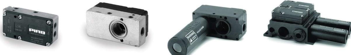
This family of pumps provides a large vacuum flow even though they are very small in size and lightweight. Vacuum level to 75 -kPa. Some pumps in this family are available with connection plate in aluminium or composite PA. These are recommended to use when the handled product is made of porous material such as cardboard, wood or paper.
