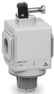
EV53 = solenoid valve, 3/2, monostable, solenoid pilot with separate air supply and bistable manual override
