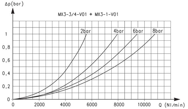
Diagram for lockable manual control valves MX3
